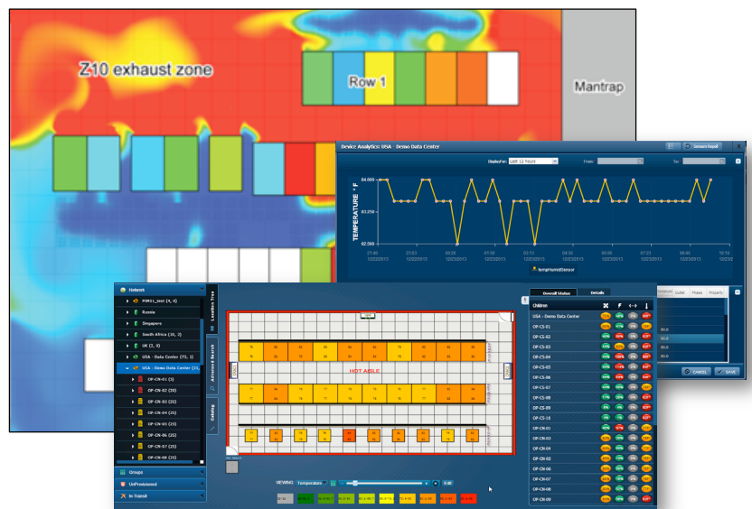
Figure 1 CFD Analysis simulates Data Center equipment with airflow and temperature
