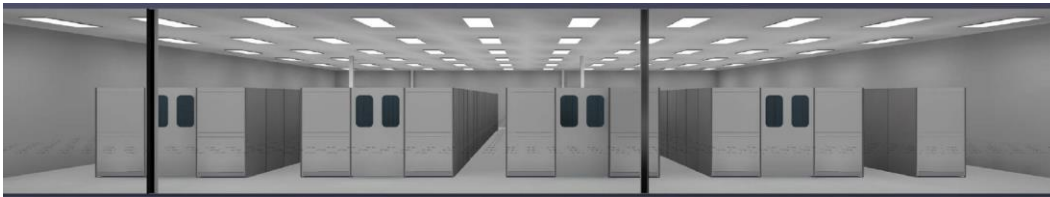
Figure 6. Model of a Data Center with White Cabinets and White Cold Aisle Containment.
