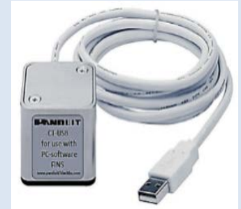
Left: The New FINS system allows for full diagnostics and record keeping of crimps and users of each tool.
