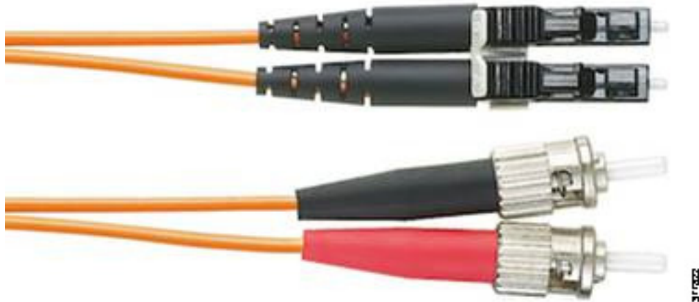
Figure 31 Hybrid Patch Cord Options—LC to ST
